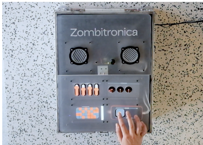
Figure 3: Zombitronica is the first prototype exploring the principle of Zombitron, made with 4 discarded smartphones and a loud-speaker.
