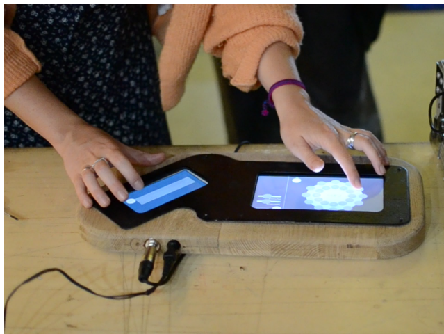
Figure 4: Zombichord is the second prototype exploring the principle of Zombitron. It was designed by Romain Segaud and Marion Jolas, inspired by the Omnichord.
