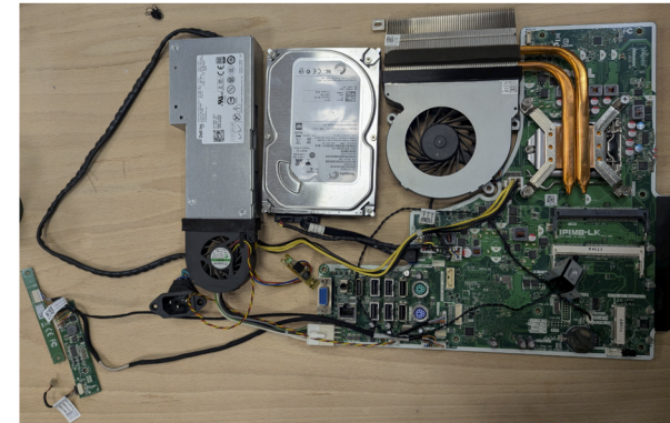
Keeping the computing part of a DELL AIO
