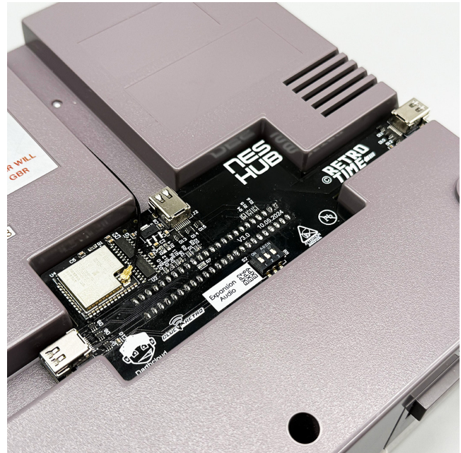
Figure 5: In 2024, modding group RetroTime released a Bluetooth adapter for the NES that plugs into an expansion port that Nintendo included but never used commercially –   8bitmods [11]
