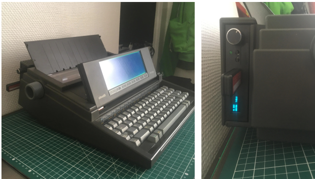
Figure 3: A Gotek floppy emulator in an Olivetti PTP820
