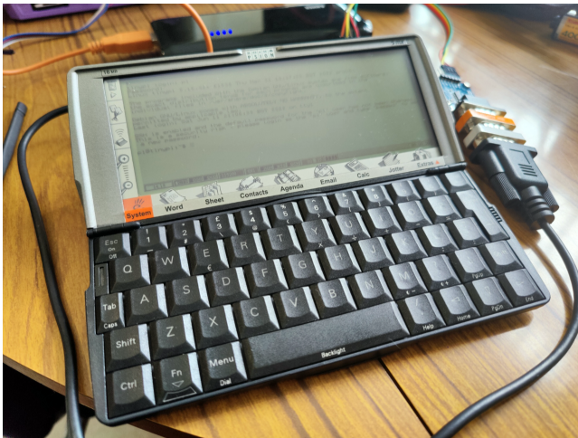
Figure 4: a Psion 5MX using a chain of adapters to connect to the internet –   Kian Ryan [23]
