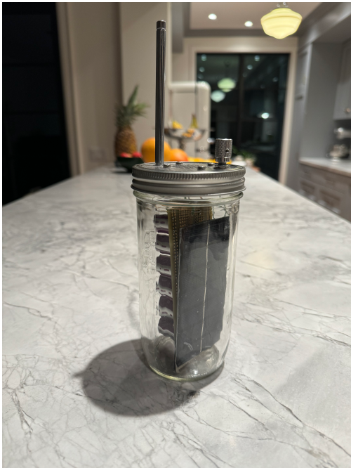
Figure 3: Open electronics FM radio in a mason jar radio with 6600F of hybrid supercapacitors in parallel - 75h of play
