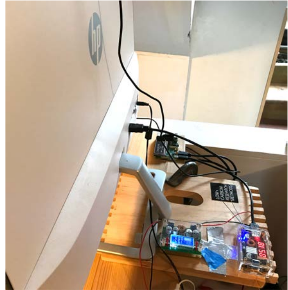
Figure 5: HP monitor, two DC-DC converters, Raspberry Pi
