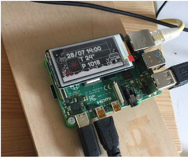
Figure 4: Raspberry Pi 4 with eInk screen
