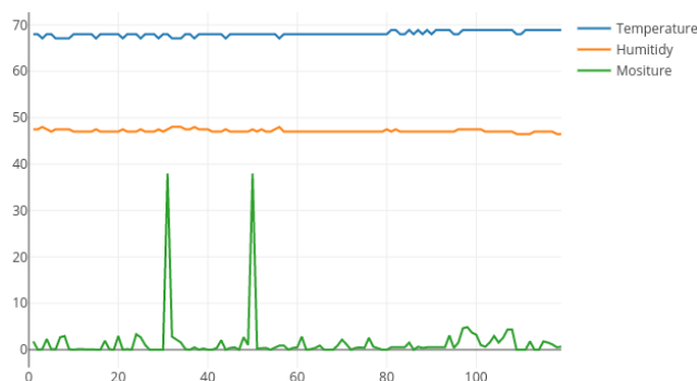
Figure 4: Sensor readings for one planter over a two hour period (created using https://plot.ly/ )
