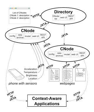
Figure 1: A diagram of the Cacophony network showing the flow of sensor data, predictions, and CNode metadata. Dashed lines are predictions being retrieved from a CNode.
